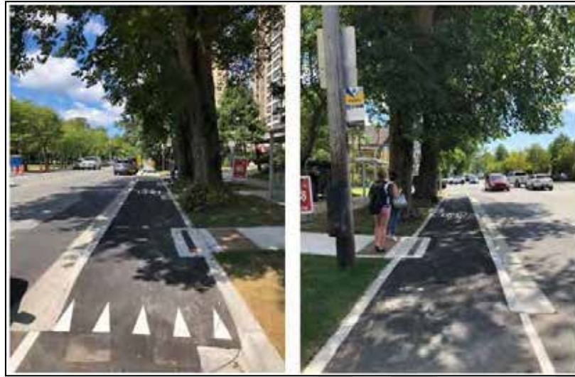
Figure 2.2.6 - Bus stop / raised bicycle lane on South Park St
